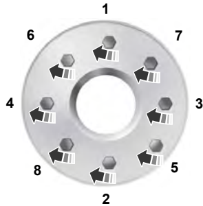
8-lug nut torque sequence
